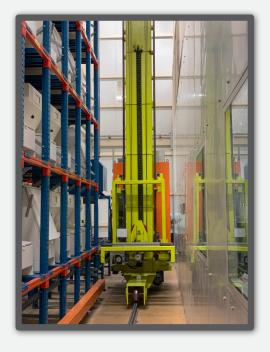
A Vertical Carousel based system stores all the required raw materials in individual bins in their designated locations. The set of raw materials required for a particular schedule will first be moved from their storage location to the batching location and arranged in their proper sequence as per the recipe.
